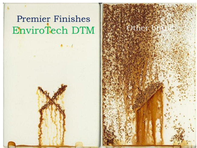
832 hours ASTM B117 Salt Fog Corrosion Resistance
