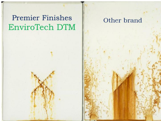
200 hours ASTM B117 Salt Fog Corrosion Resistance
